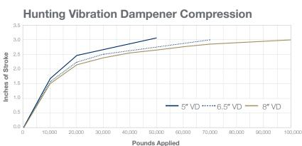
The 5-in. Vibration Dampener's 50,000-lb maximum rating; the 6.5-in. Vibration Dampener's 70,000-lb maximum rating and the 8-in. Vibration Dampener's 100,000-lb maximum rating will compress the tool 3 in.
